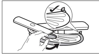
7. Reassemble the filters (B) and (C).
