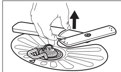
2. Wash the spray arm under running water. Use a thin pointed tool, e.g. a toothpick, to remove particles of soil from the holes. Run water through the holes to wash soil particles away from the inside.
