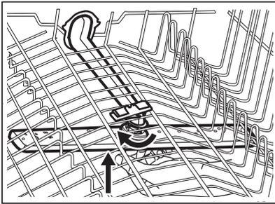
3. Wash the spray arm under running water. Use a thin pointed tool, e.g. a toothpick, to remove particles of soil from the holes. Run water through the holes to wash soil particles away from the inside.
